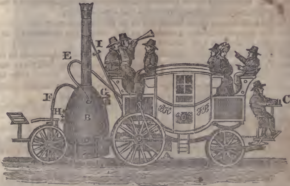
A, Water Cistern—B, the Boiler—C, Steering Wheel with the Conductor—D, Steel Frame which carries the Boiler—E, the Curved Steam Pipe to supply the Engines—F, Hand Pump and Pipe to fill the Boiler—G, Safety Valve—H, Notice Cocks—I, Eduction Pipe to take the steam from the Engine to the Chimney—K, the Crank—L, the Fan for the Cinders.
